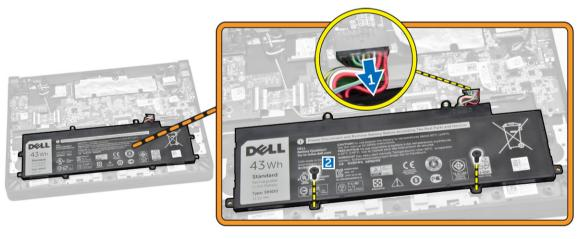
3. Lift the battery and remove it from the computer.
